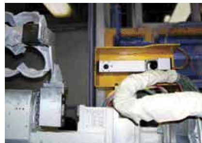
FIGURE 2. SICK IVC-3D 200 unit compiles a 3-D surface map of the core from thousands of 2-D laser profiles.
